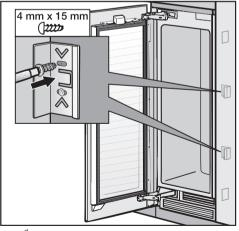
Secure the retaining clips for the space covers on both sides.
